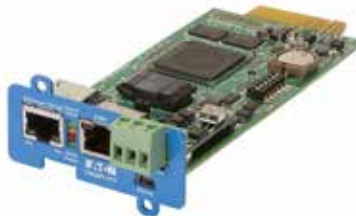
Figure 5-5: PowerXpert UPS MiniSlot card (PXGMS UPS)
